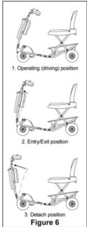
**CAUTION:** When getting in and out of the **EasyTravel** seat, step only on **CENTER** of foot platform. **DO NOT STEP ON SIDE OF FOOT PLATFORM** to avoid tipping the **EasyTravel**.
